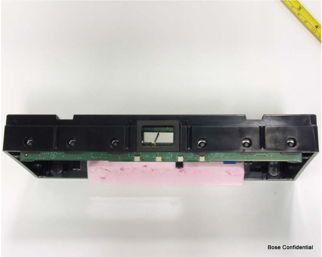
Antenna location in case top
