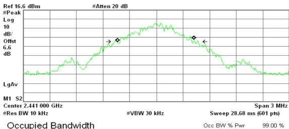
Occupied Bandwidth 857.8137 kHz Occ BVV % Pwr 99.00 % x dB -20.00 dB
