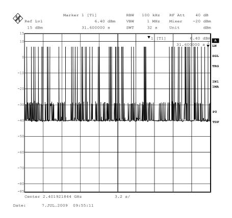
There are 58 pulses in 31.6 seconds. Therefore the average dwell time per channel is 0.634 ms x 58 = 36.7 ms which is less than the allowed 400ms.
