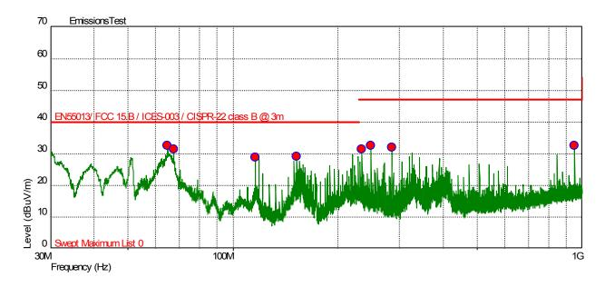
Legend: Green: Automated peak detector readings Red dots: Indicate highest recorded peaks using max peak detector
