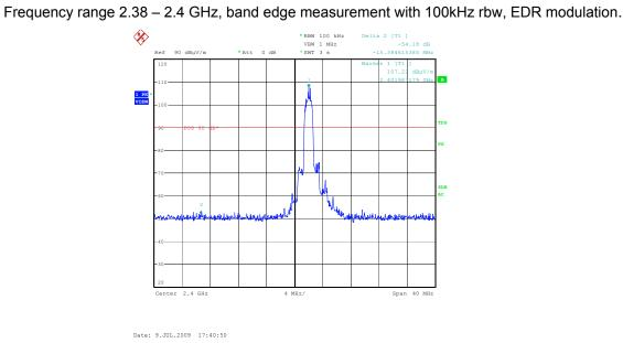
The delta between the in-band and the maximum value in the lower adjacent restricted band is 54.18 dB Actual peak and average measured in-band value with 1 MHz rbw and basic rate modulation
