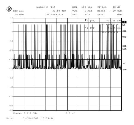
There are 64 pulses in 31.6 seconds. Therefore the average dwell time per channel is 0.634 ms x 64 = 40.6 ms which is less than the allowed 400ms.
