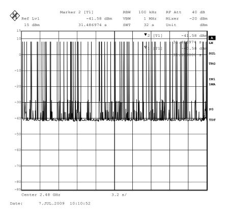
There are 67 pulses in 31.6 seconds. Therefore the average dwell time per channel is 0.634 ms x 67 = 42.5 ms which is less than the allowed 400ms.
