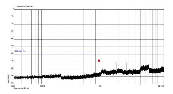
Max level @ 927.95MHz is - 68.44 dBm or 0.14 nW
