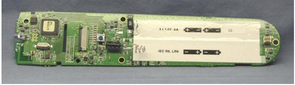
Bottom of circuit board – button contact area
