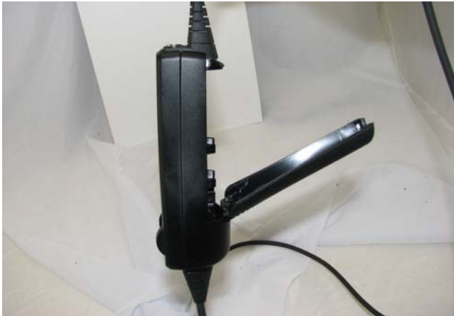
Side-view of tethered battery compartment
