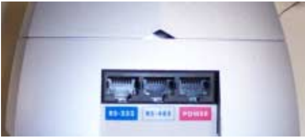
Figure 2: Reader RS232, RS485 and Power Connectors
