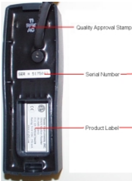
Figure 2. Backside of Mullion with back plate removed
