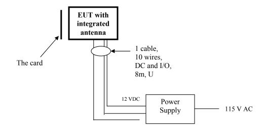
Note: Two I/O wires, green and orange, are connected together, all others are open.
