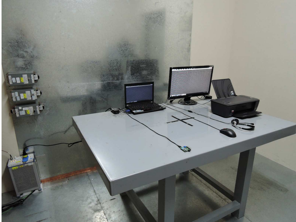
Photograph 6: Set-up for for Mains Conducted testing Front
