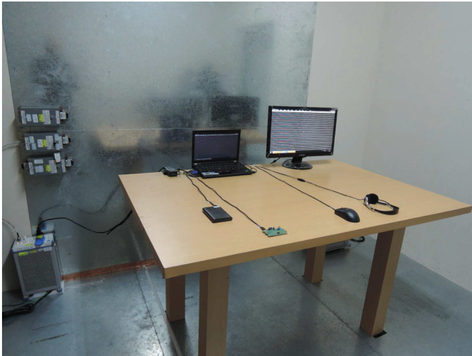
Photograph 6: Set-up for for Mains Conducted testing Front
