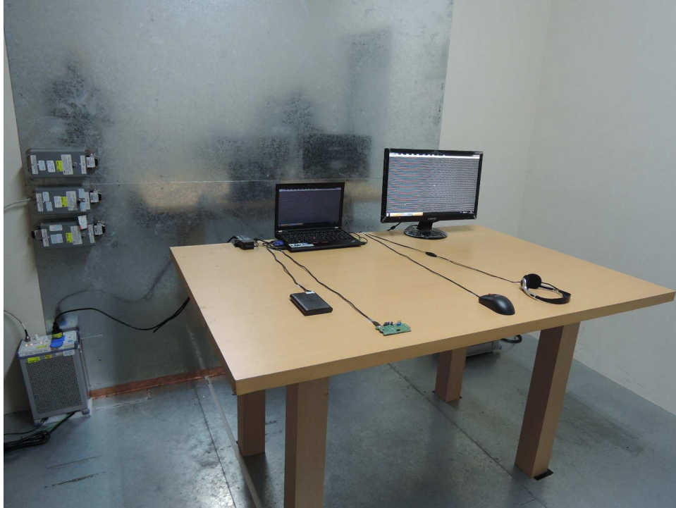
Photograph 6: Set-up for for Mains Conducted testing Front
