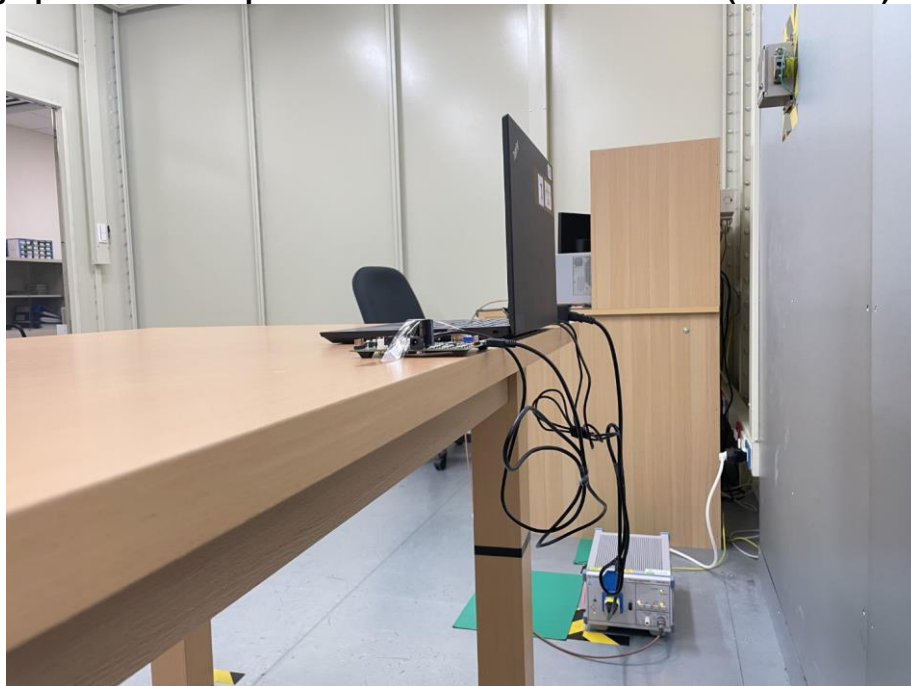
Photograph 8: Test Setup for Mains Conducted Emissions (Back View)
