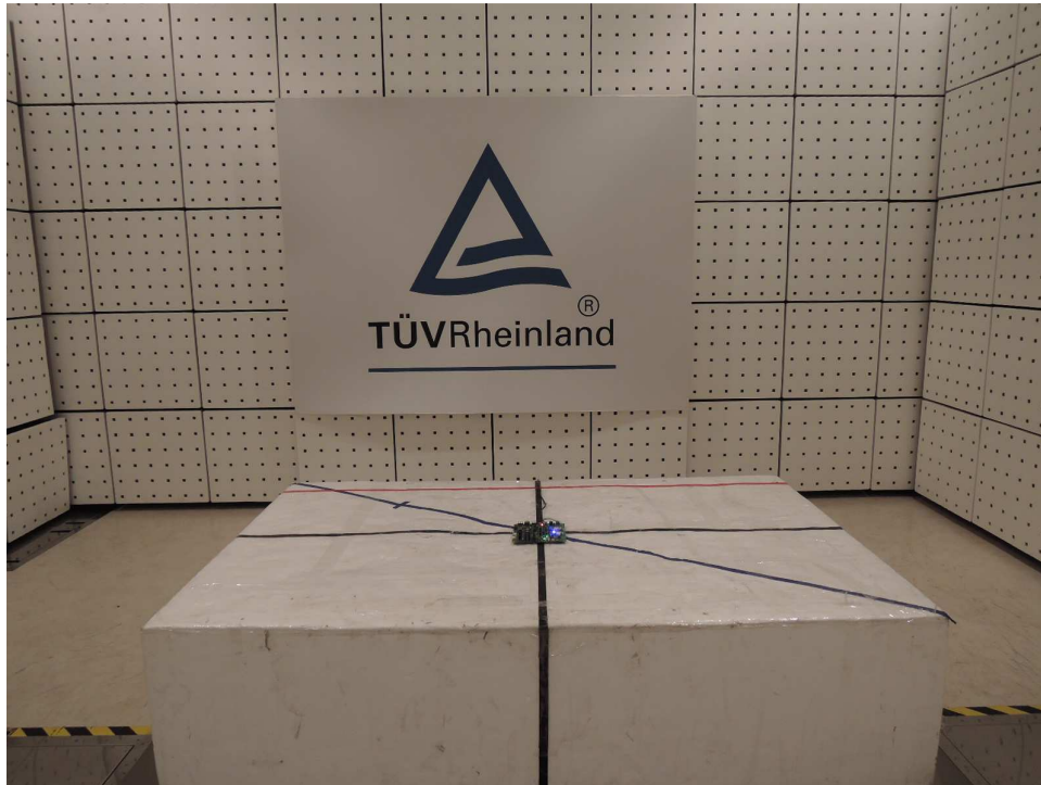
Photograph 2: Set-up for Spurious Emissions (Back View 1)
