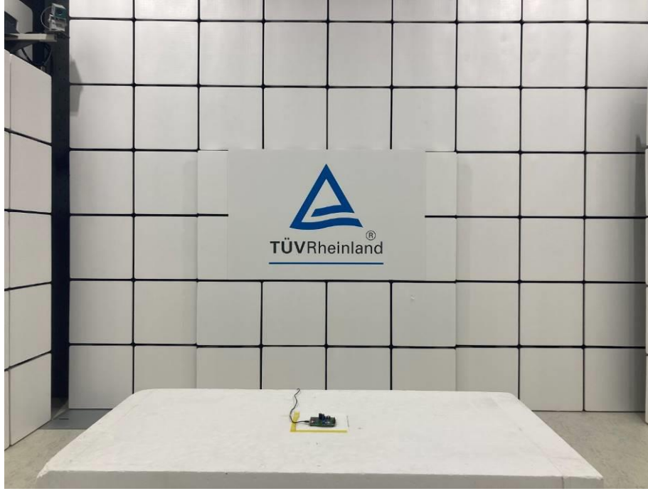
Photograph 2: Test Setup for Spurious Emissions (Front View 2)
