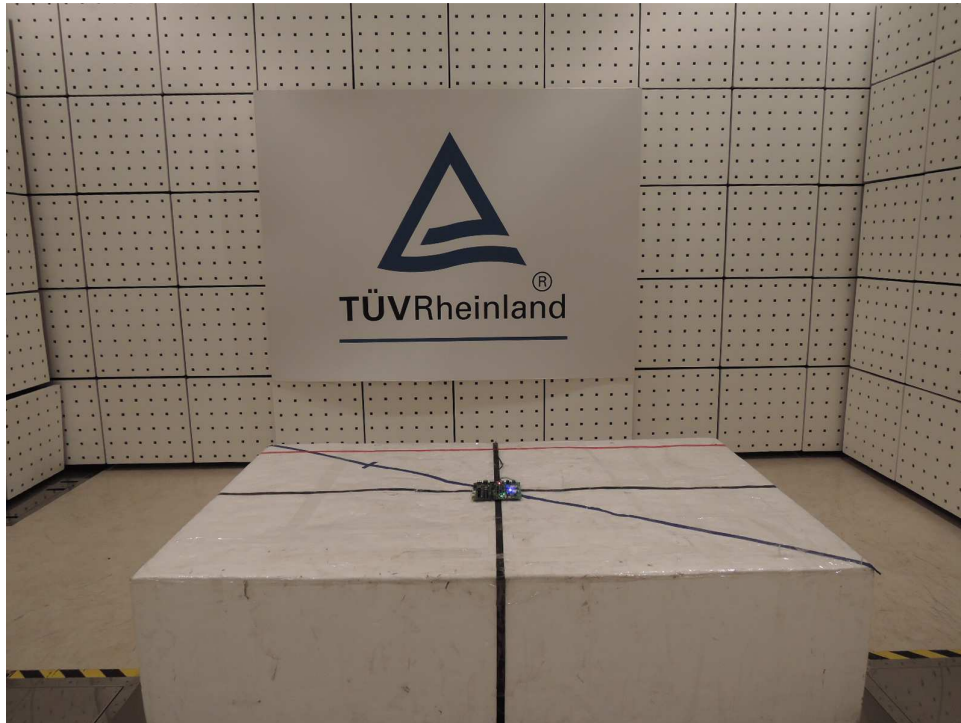
Photograph 2: Set-up for Spurious Emissions (Back View 1)
