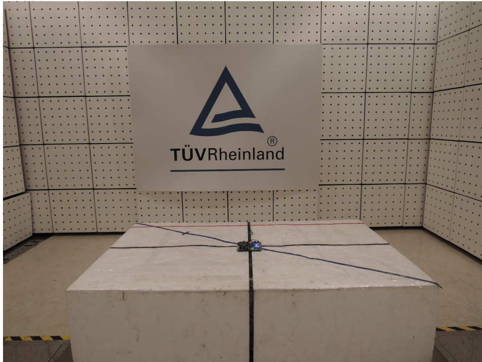
Photograph 1: Set-up for Spurious Emissions (Front View)
