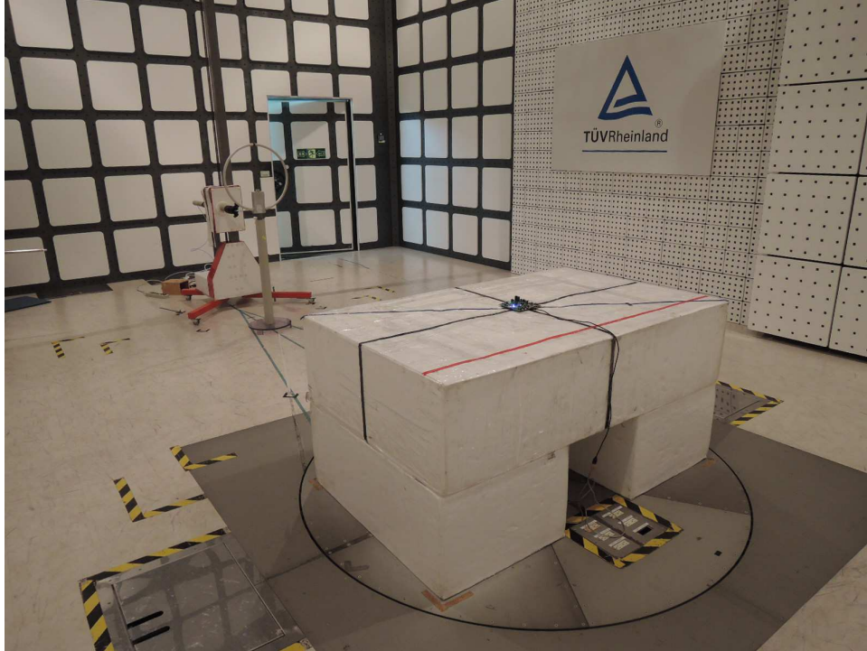
Photograph 3: Set-up for Spurious Emissions (Back View 2)
