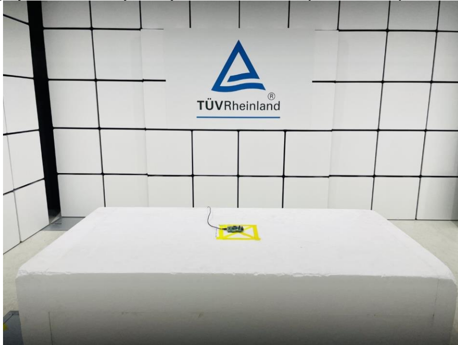
Photograph 2: Test Setup for Spurious Emissions (Front View 2)
