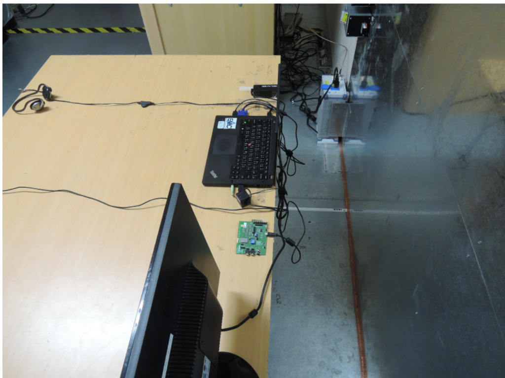
Photograph 5: Set-up for for Mains Conducted testing Back
