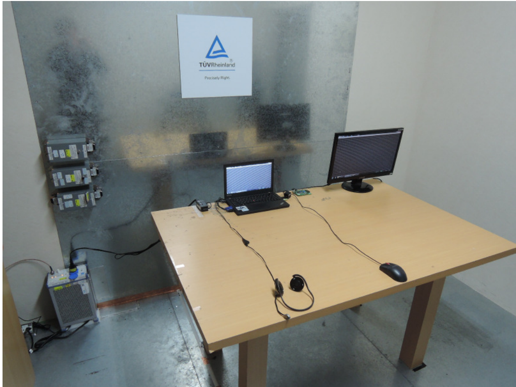
Photograph 6: Set-up for for Mains Conducted testing Front
