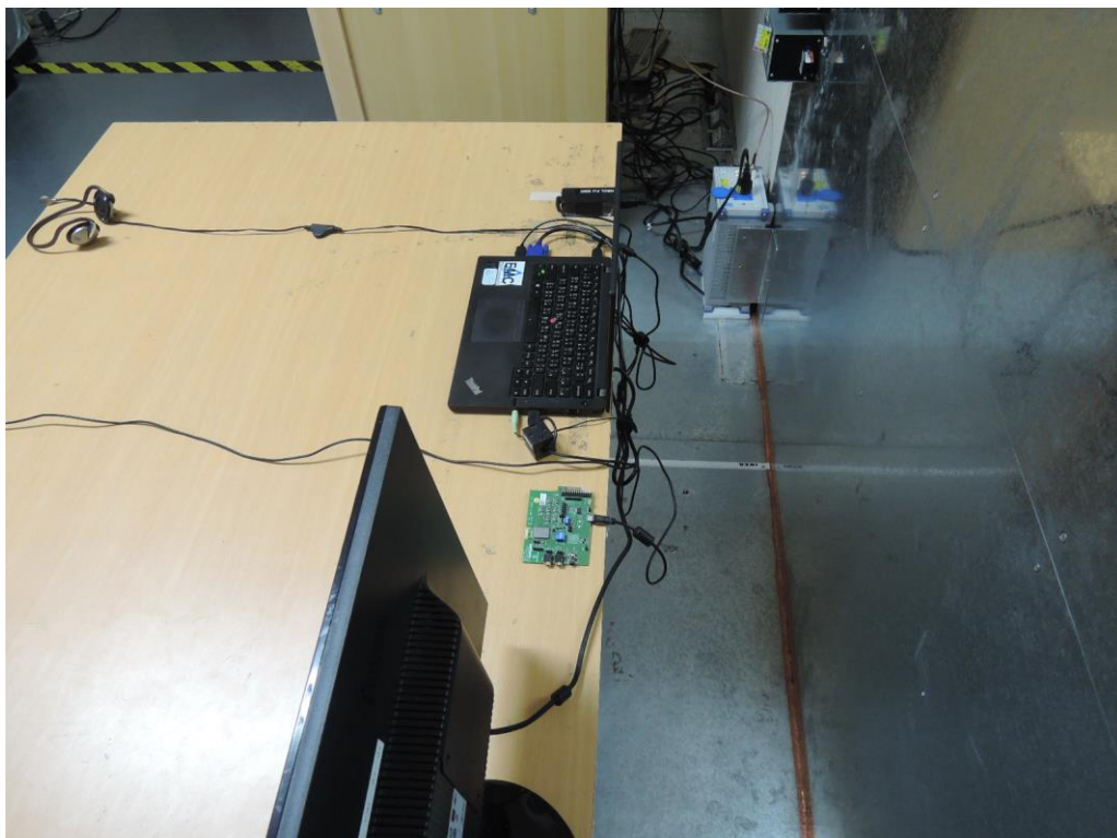
Photograph 5: Set-up for for Mains Conducted testing Back
