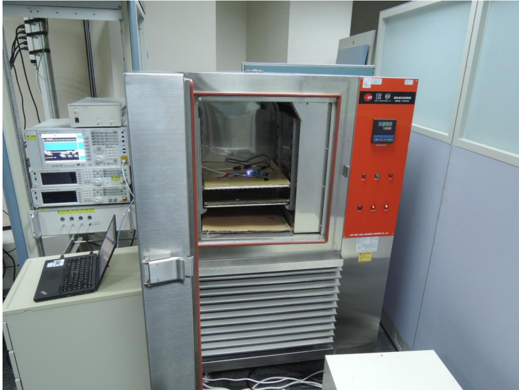
Photograph 5: Set-up for for Mains Conducted testing Back
