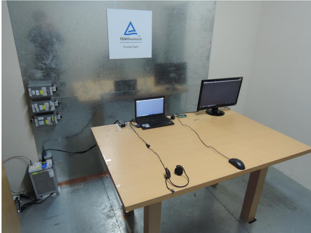
Photograph 6: Set-up for for Mains Conducted testing Front
