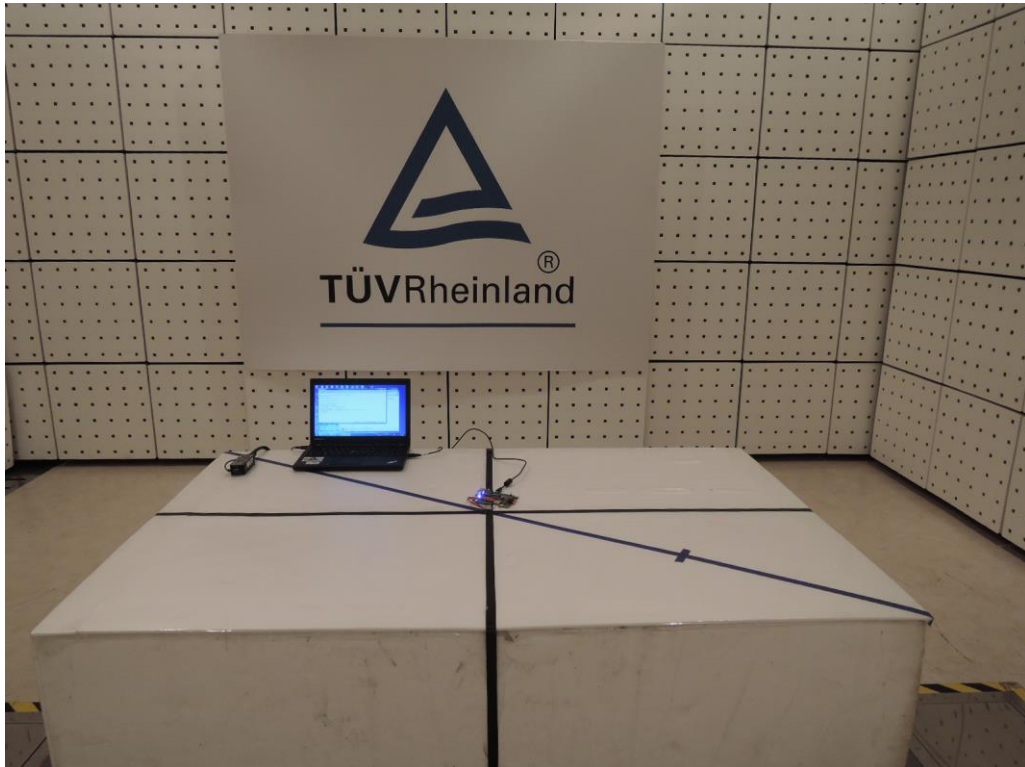
Photograph 1: Set-up for Spurious Emissions (Front View)
