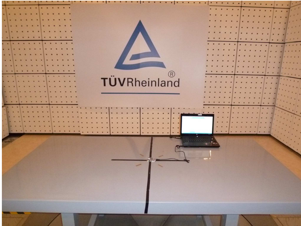
Photograph 2: Set-up for Spurious Emissions (Back View)
