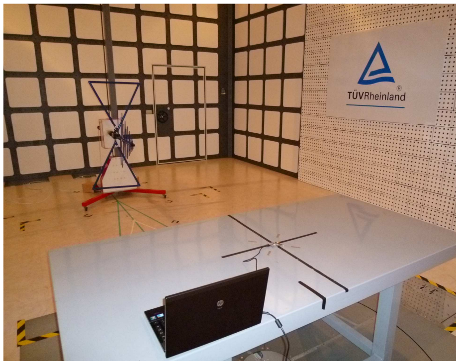
Photograph 2: Set-up for Spurious Emissions (Back View)
