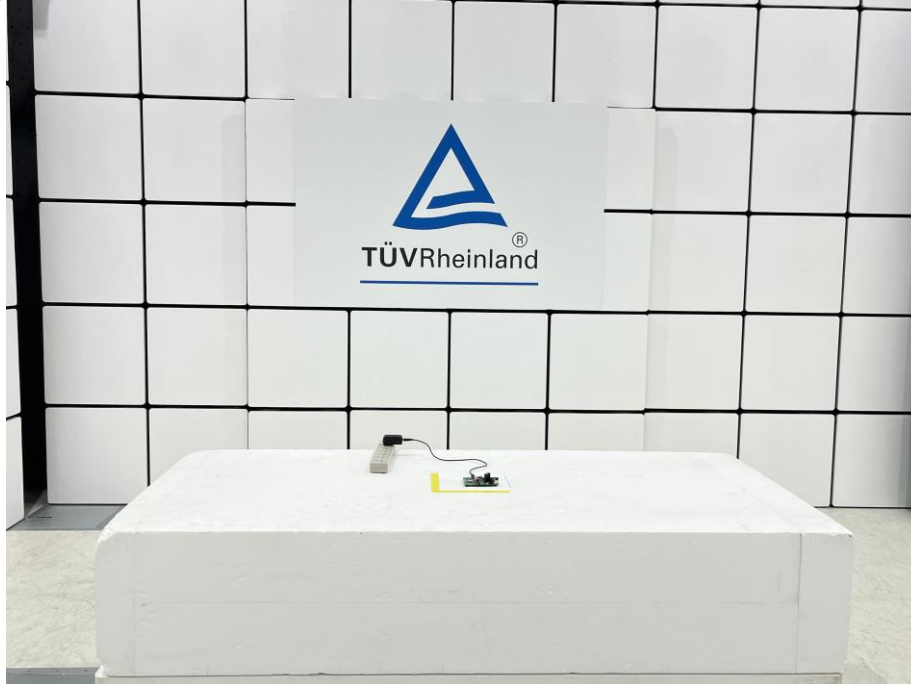
Photograph 2: Test Setup for Spurious Emissions (Front View 2)
