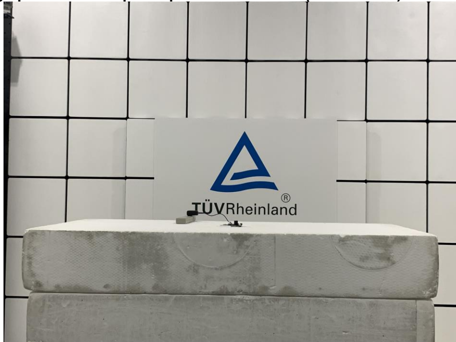
Photograph 2: Test Setup for Spurious Emissions (Front View 2)
