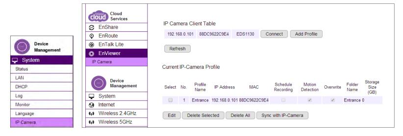
**Note: Only EnGenius Cameras** can be managed collectively by EnGenius Gateway/Router. For other vendor's cameras, you still have to configure them one by one manually.
