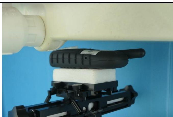
Rear Face of Short Ant Tested at 10 mm
