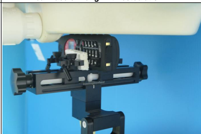
Right Side of Long Ant Tested at 0 mm
