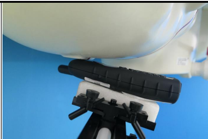
Right Tilted of Short Ant Tested
