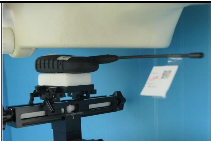
Rear Face of Long Ant Tested at 10 mm
