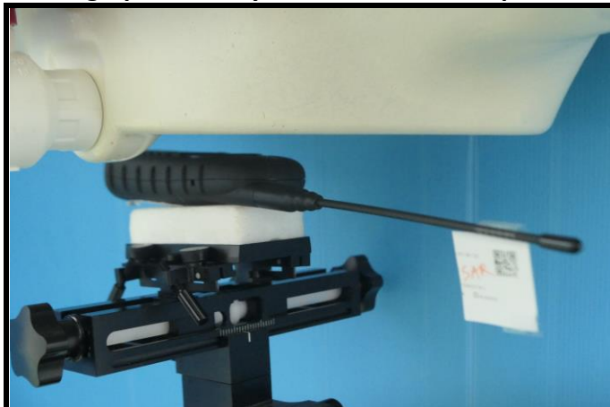
Front Face of Long Ant Tested at 10 mm
