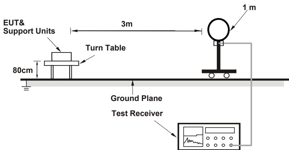
**For Radiated emission 30MHz to 1GHz**
