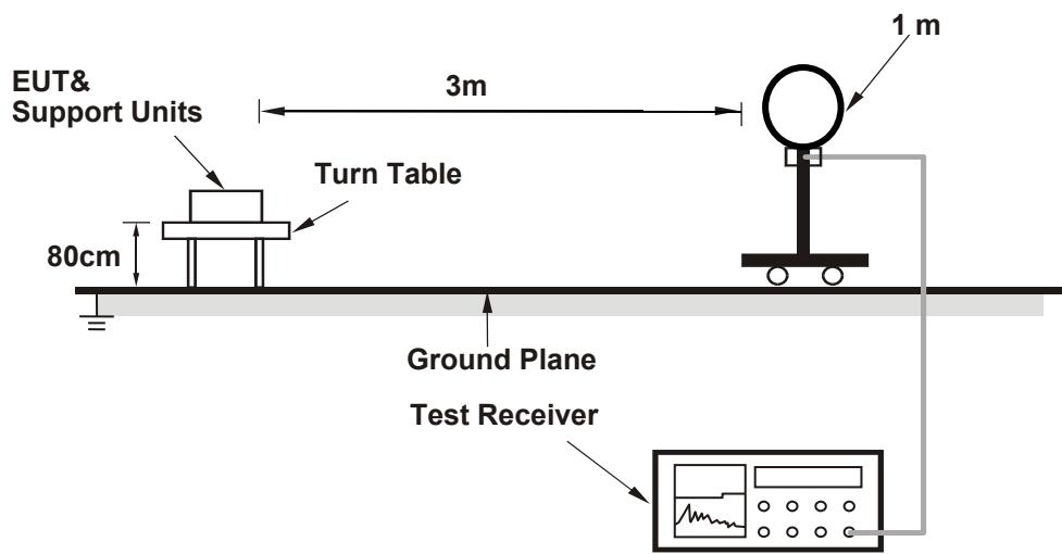
**For Radiated emission 30MHz to 1GHz**
