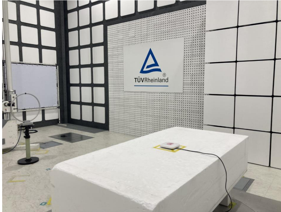
Photograph 22: Test Setup for Spurious Emissions (Back View 2, POE Mode)
