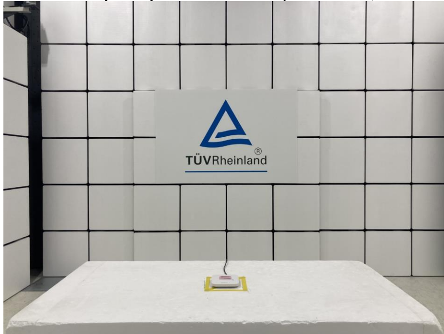
Photograph 20: Test Setup for Spurious Emissions (Front View 2, POE Mode)
