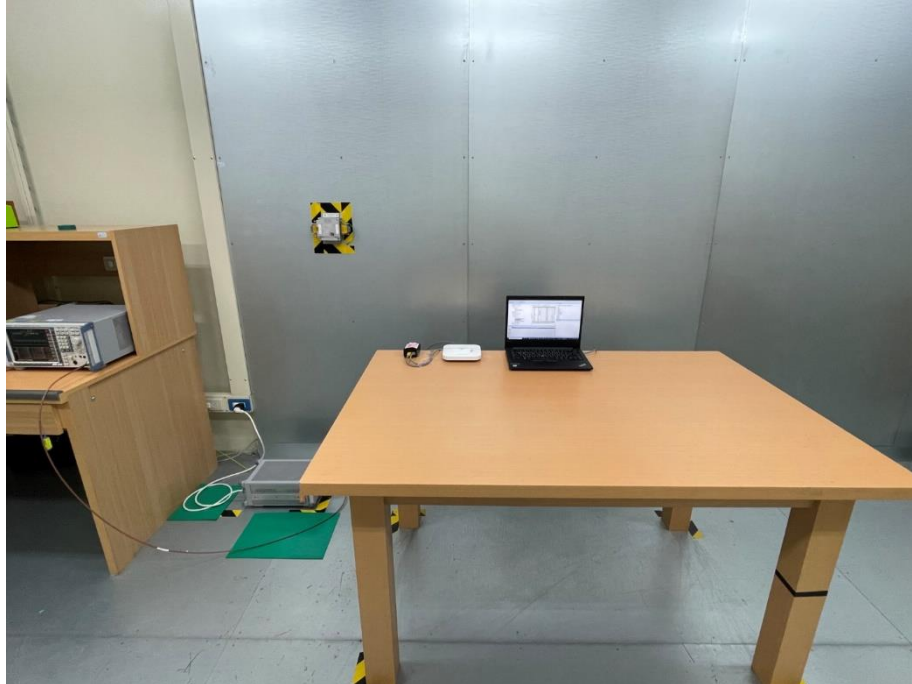
Photograph 28: Test Setup for Mains Conducted Emissions (Back View, POE Mode)
