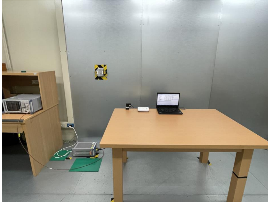
Photograph 26: Test Setup for Mains Conducted Emissions (Back View, Adapter Mode)
