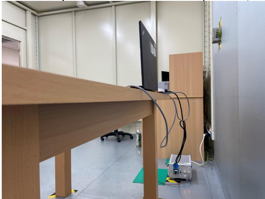
Photograph 28: Test Setup for Mains Conducted Emissions (Back View, POE Mode)
