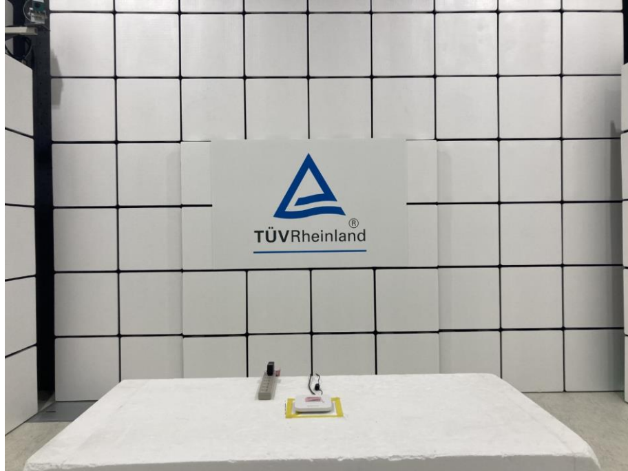
Photograph 13: Test Setup for Spurious Emissions (Front View 1, Adapter Mode)
