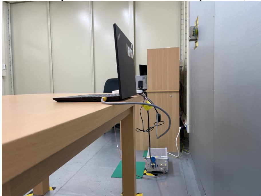
Photograph 26: Test Setup for Mains Conducted Emissions (Back View, Adapter Mode)
