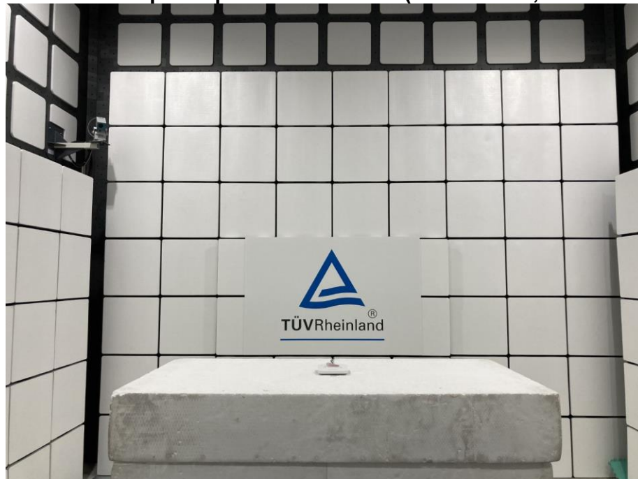
Photograph 20: Test Setup for Spurious Emissions (Front View 2, POE Mode)
