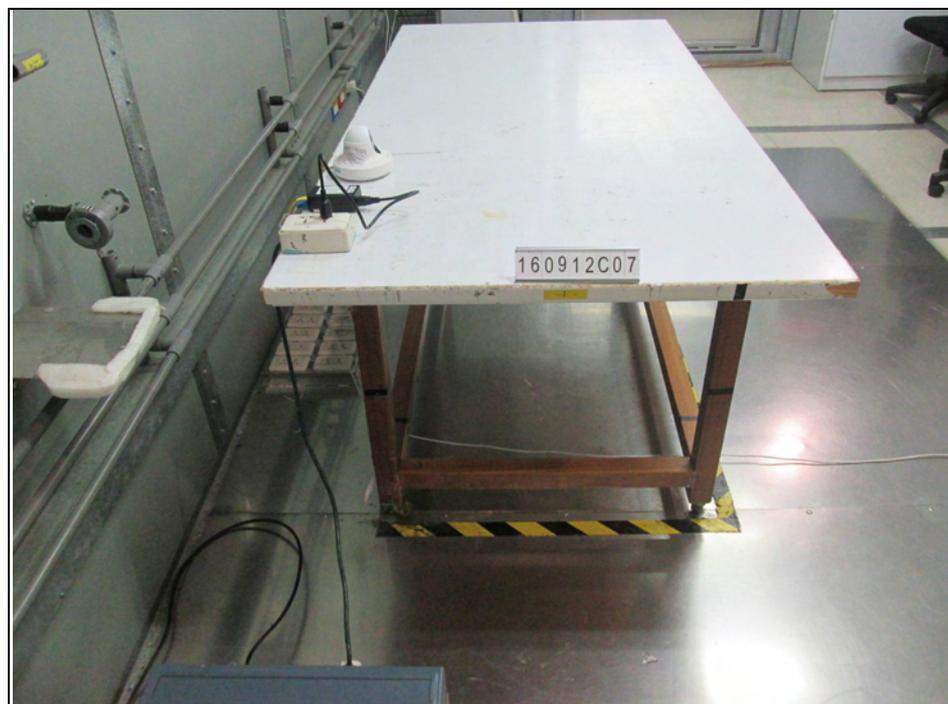
RADIATED EMISSION TEST (Frequency above 1GHz)
