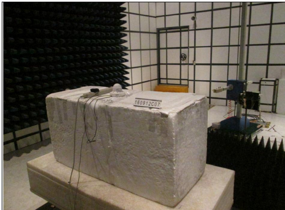
RADIATED EMISSION TEST (Frequency above 1GHz)
