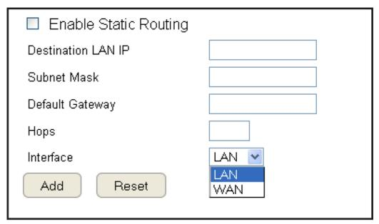
Click **Add** to save the settings and list the configuration in the Current Static Routing table or **Reset** the discard changes.
