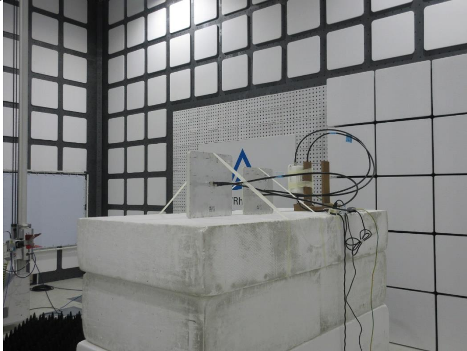
Photograph 11: Test Setup for Spurious Emissions (Back View 3)
