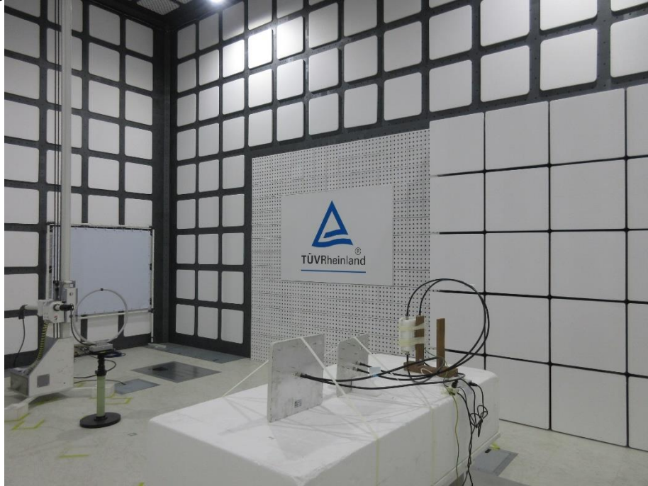
Photograph 9: Test Setup for Spurious Emissions (Back View 1)
