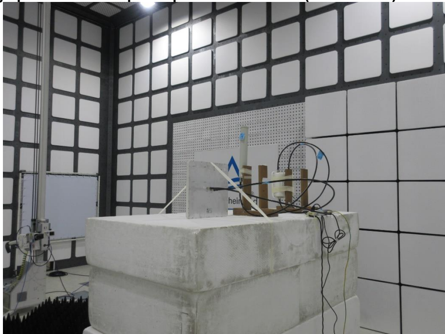
Photograph 18: Test Setup for Spurious Emissions (Back View 4)
