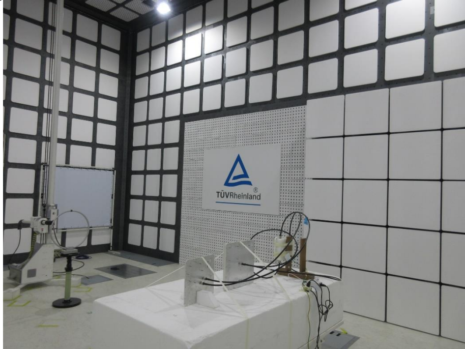
Photograph 21: Test Setup for Spurious Emissions (Back View 1)
