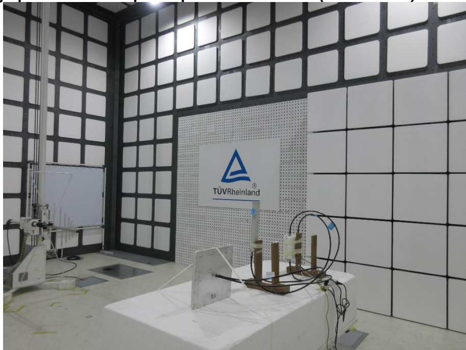
Photograph 16: Test Setup for Spurious Emissions (Back View 2)
