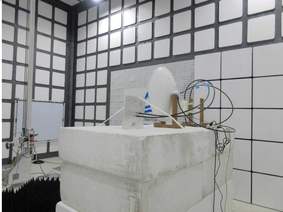
Photograph 29: Test Setup for Spurious Emissions (Back View 3)
