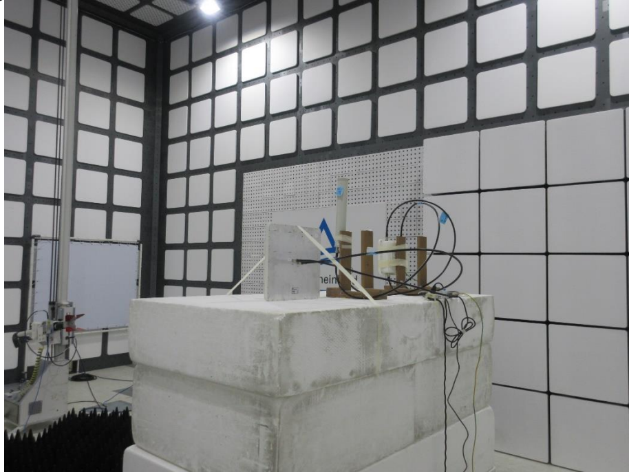
Photograph 17: Test Setup for Spurious Emissions (Back View 3)
