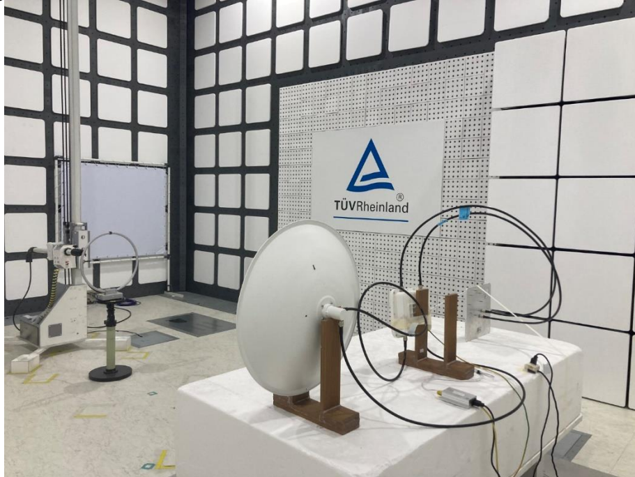
Photograph 3: Test Setup for Spurious Emissions (Back View 1)
