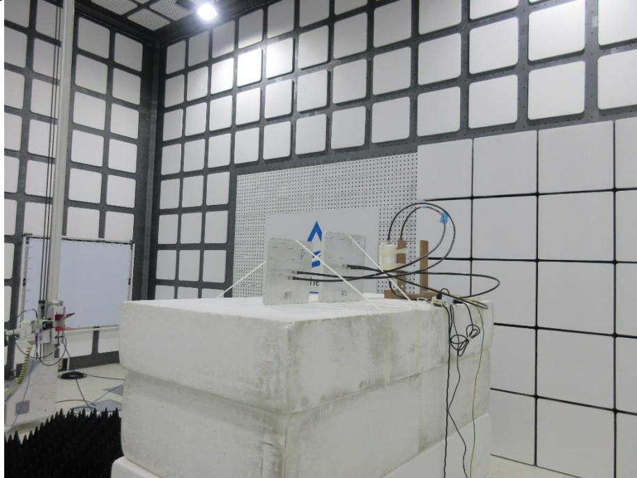
Photograph 23: Test Setup for Spurious Emissions (Back View 3)
