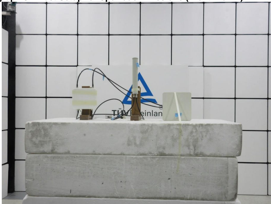
Photograph 32: Test Setup for Spurious Emissions (Front View 2)
