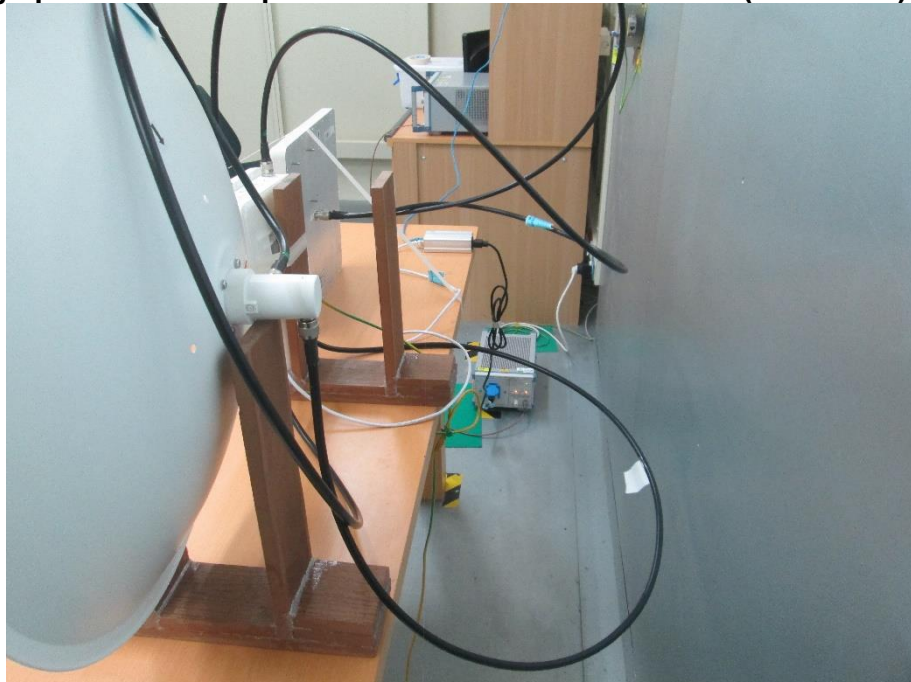
Photograph 38: Test Setup for Mains Conducted Emissions (Back View)
