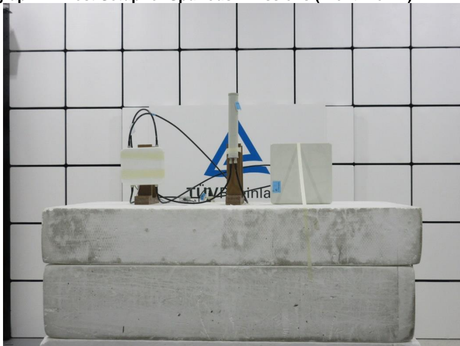
Photograph 14: Test Setup for Spurious Emissions (Front View 2)
