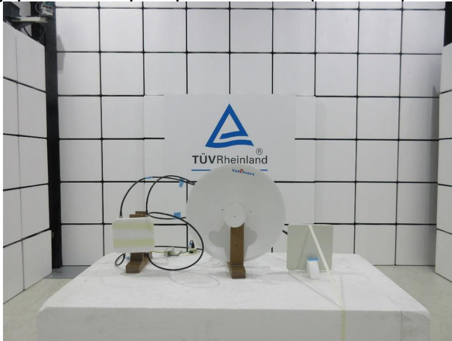
Photograph 26: Test Setup for Spurious Emissions (Front View 2)
