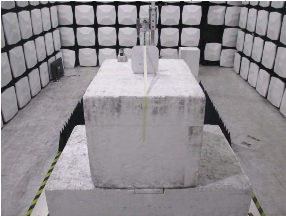
Description : Rear View of Radiated Emission Test Setup (Above 1 GHz)
