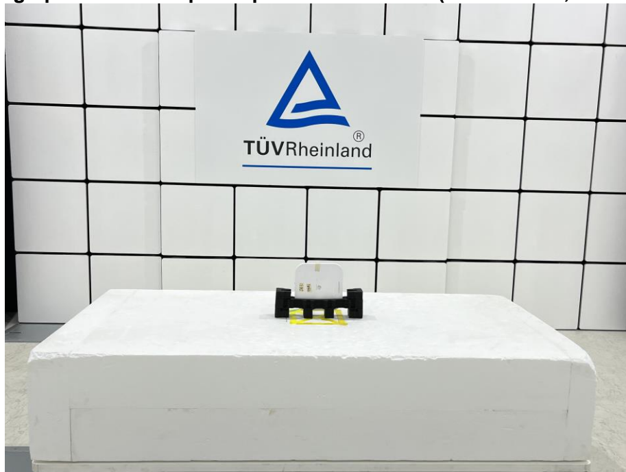
Photograph 10: Test Setup for Spurious Emissions (Front View 2, POE Mode)
