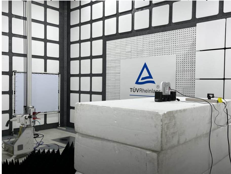
Photograph 6: Test Setup for Spurious Emissions (Back View 4, Adapter Mode)
