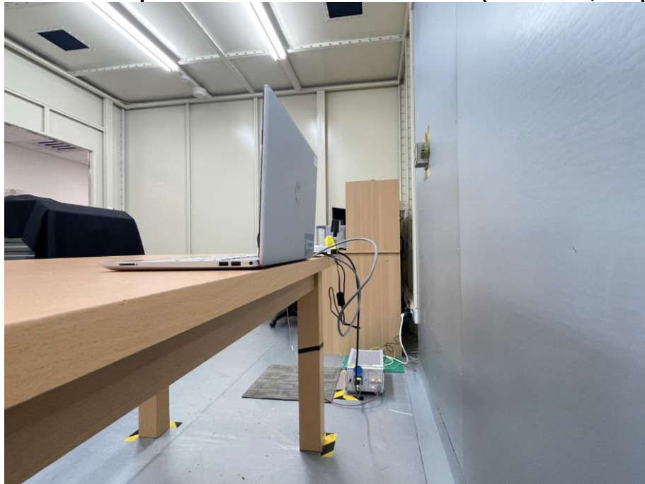
Photograph 8: Test Setup for Mains Conducted Emissions (Back View, Adapter Mode)
