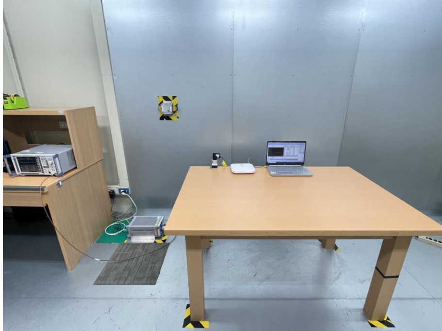
Photograph 8: Test Setup for Mains Conducted Emissions (Back View, Adapter Mode)
