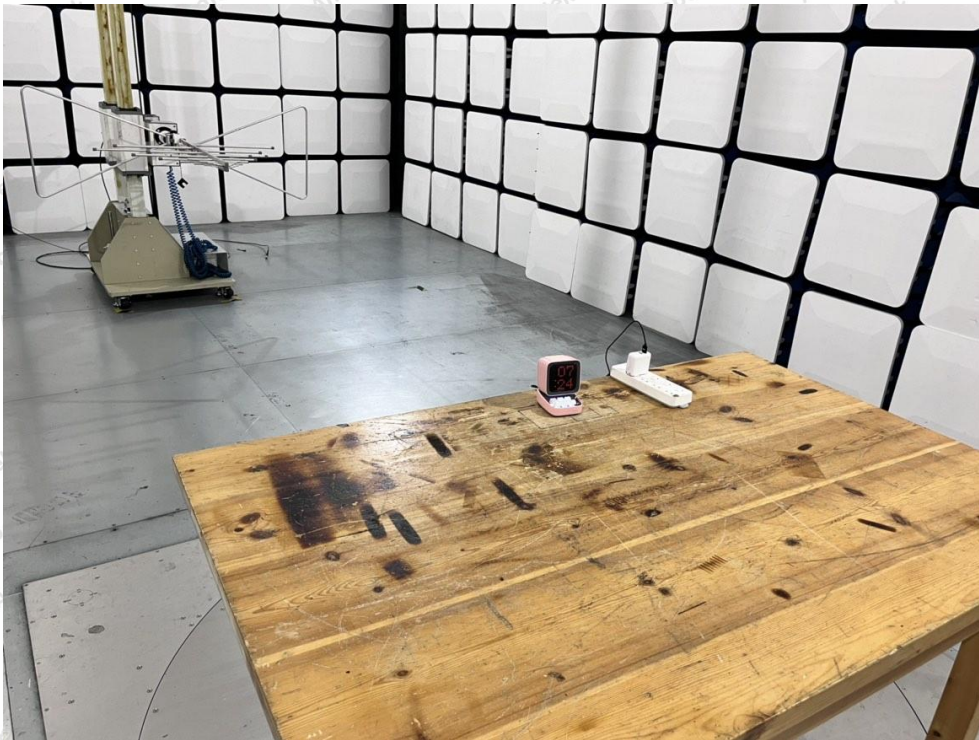
Photo of Radiation Emission Test
