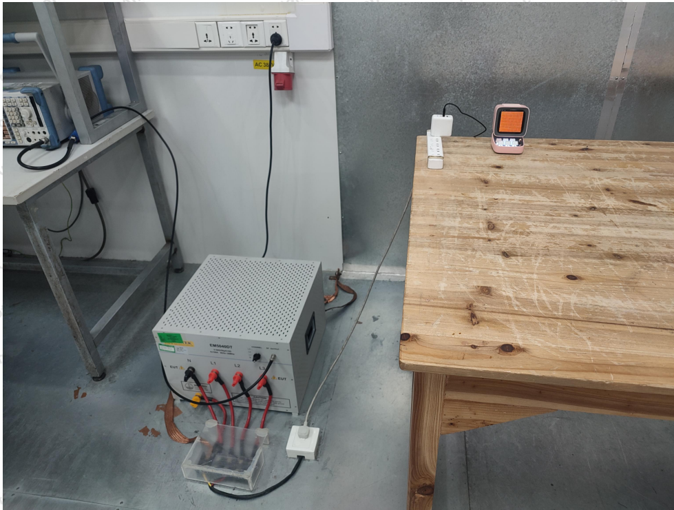
Photo of Conducted Emission Measurement
