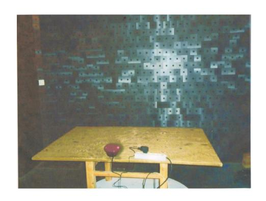
RADIATED EMISSION TEST ABOVE 1GHz
