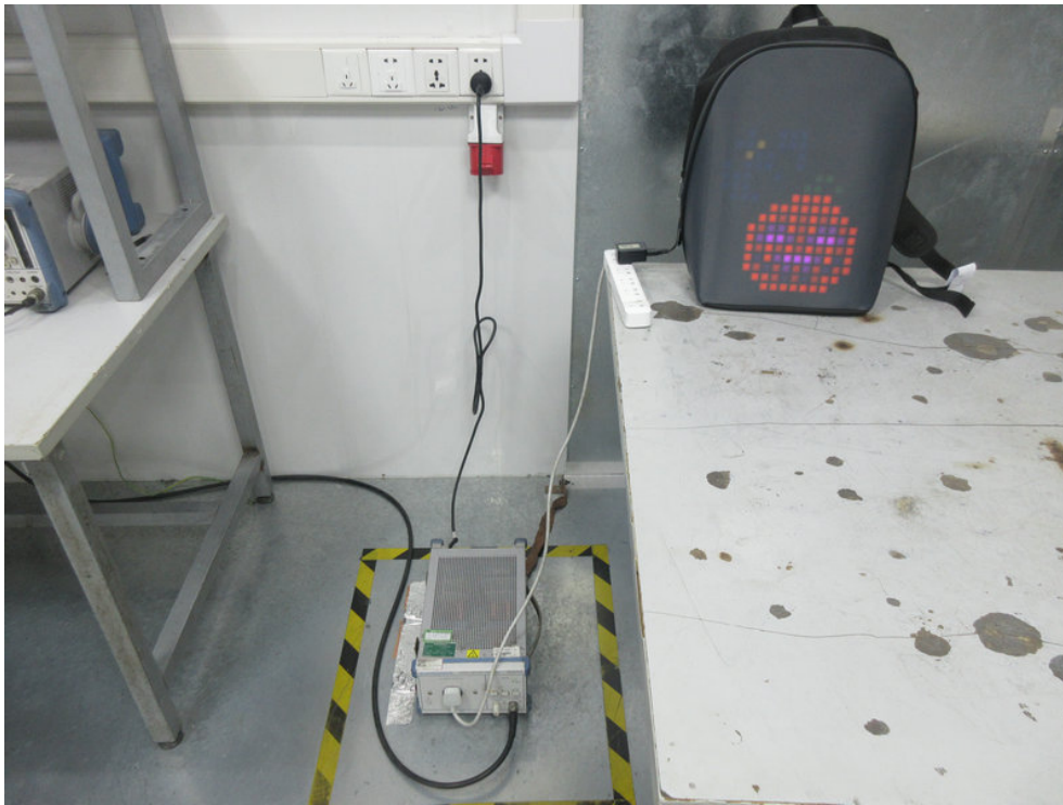
Photo of Radiation Emission Test
