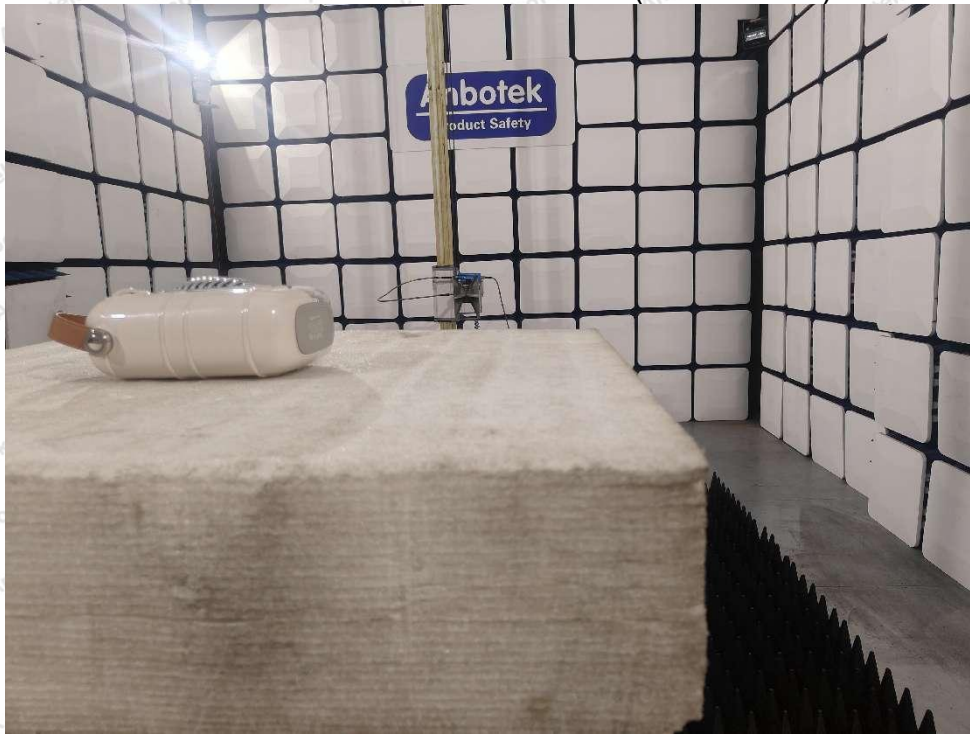
Photo of Radiation Emission Test (above 1GHz)
