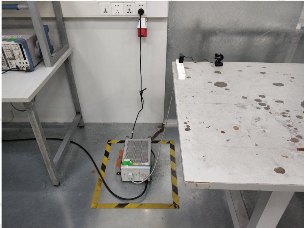
Photo of Conducted Emission Measurement
