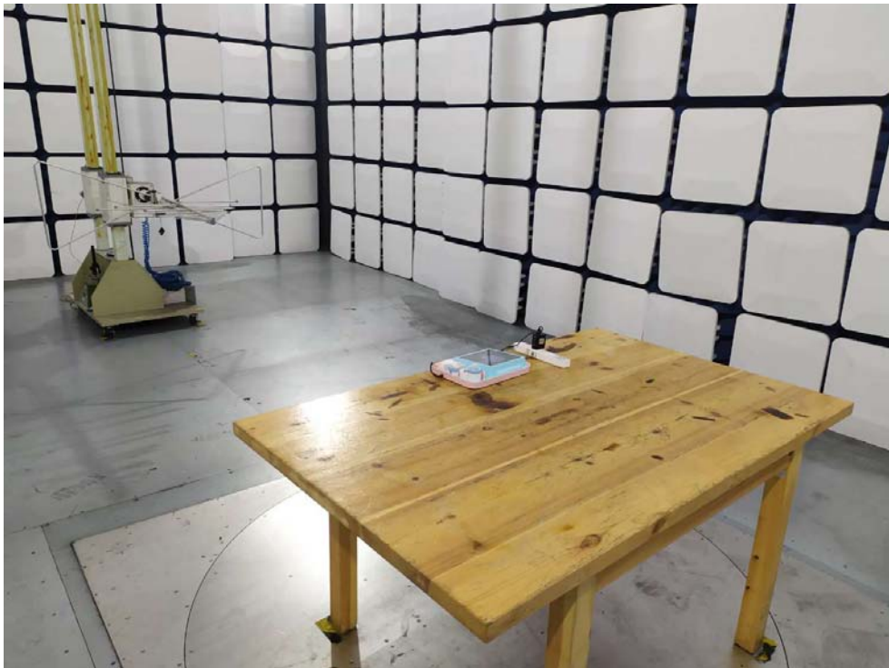
Photo of Radiation Emission Test
