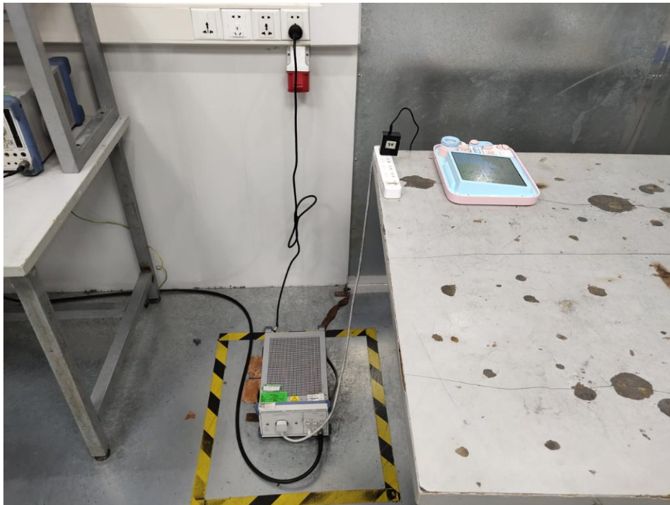
Photo of Radiation Emission Test
