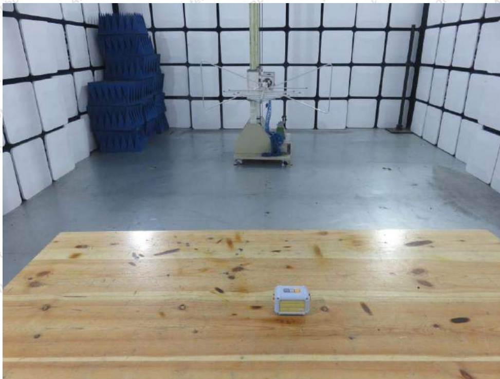
Photo of Radiation Emission Test
