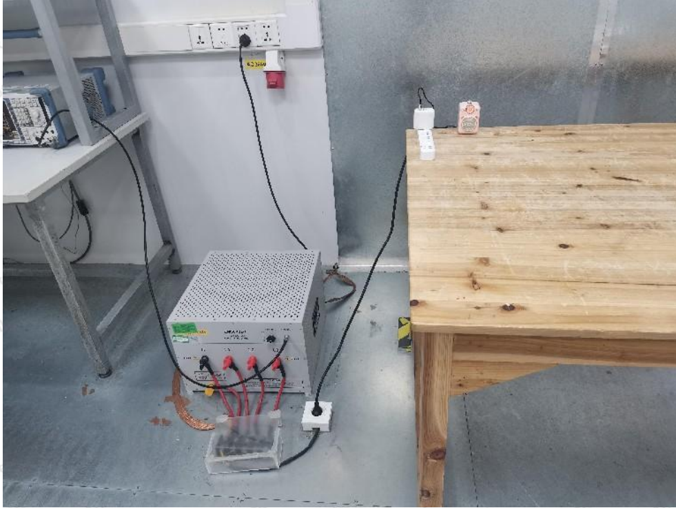
Photo of Conducted Emission Measurement
