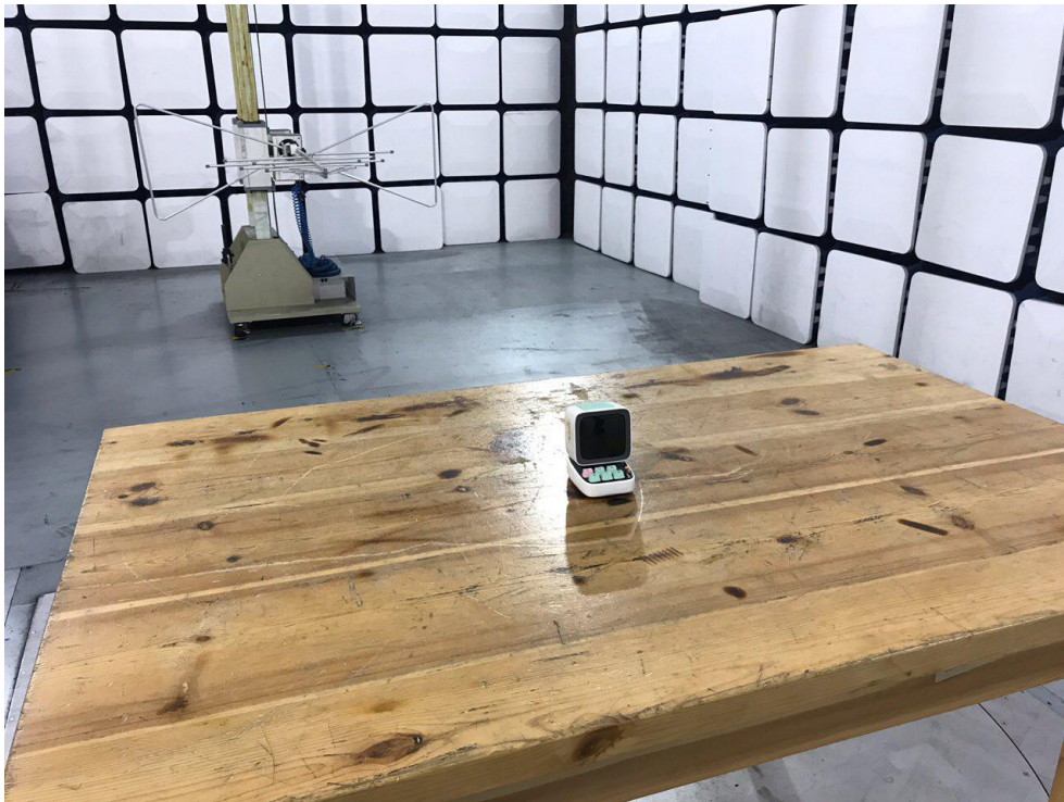
Photo of Radiation Emission Test
