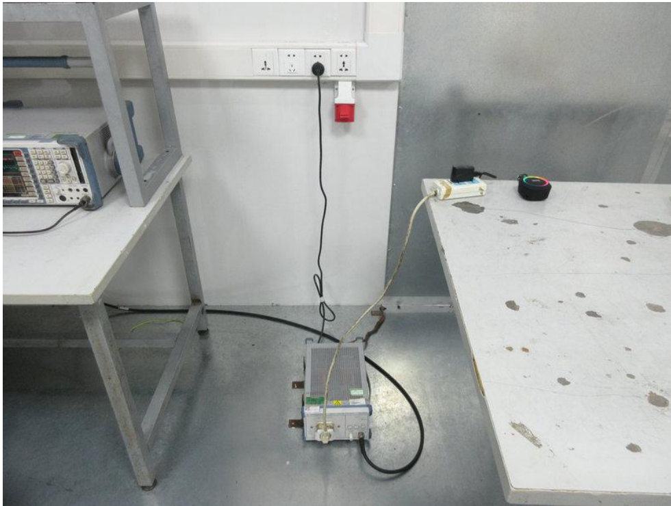
Photo of Conducted Emission Test
