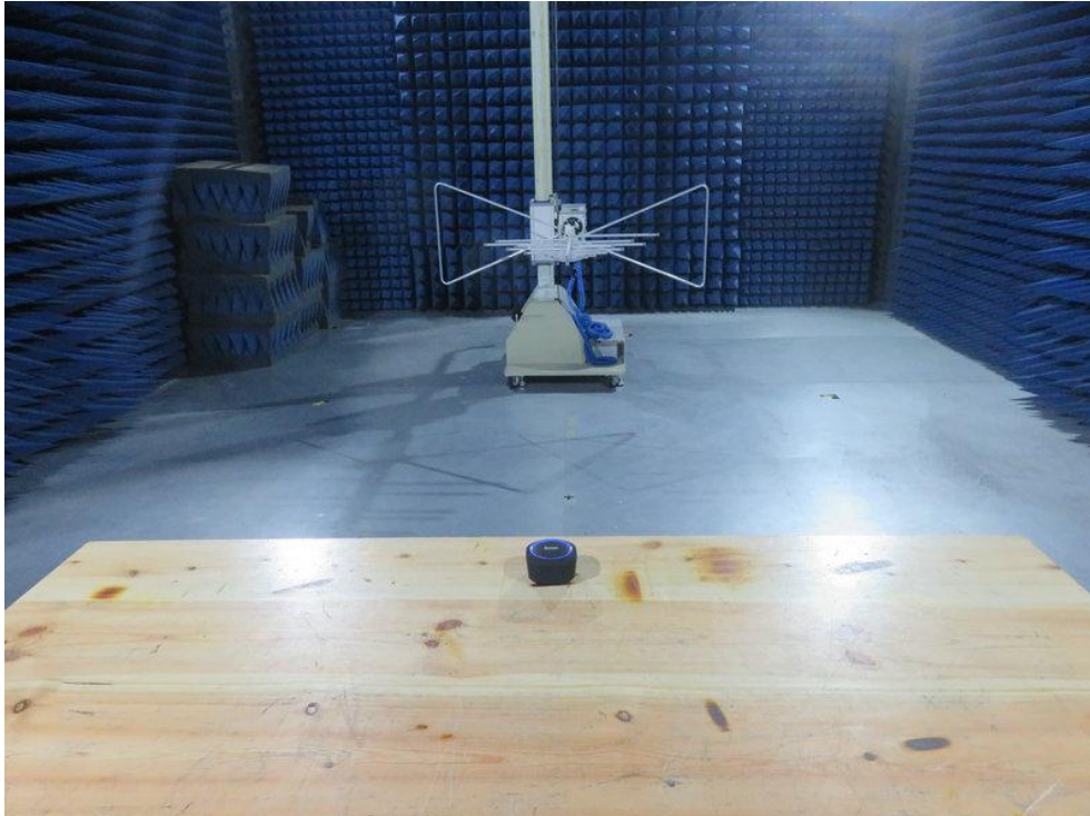
Photo of Radiation Emission Test
