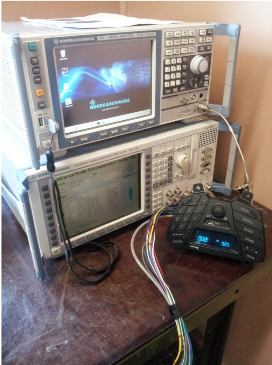
Figure 5: Conducted RF Test Setup Photograph(s).
