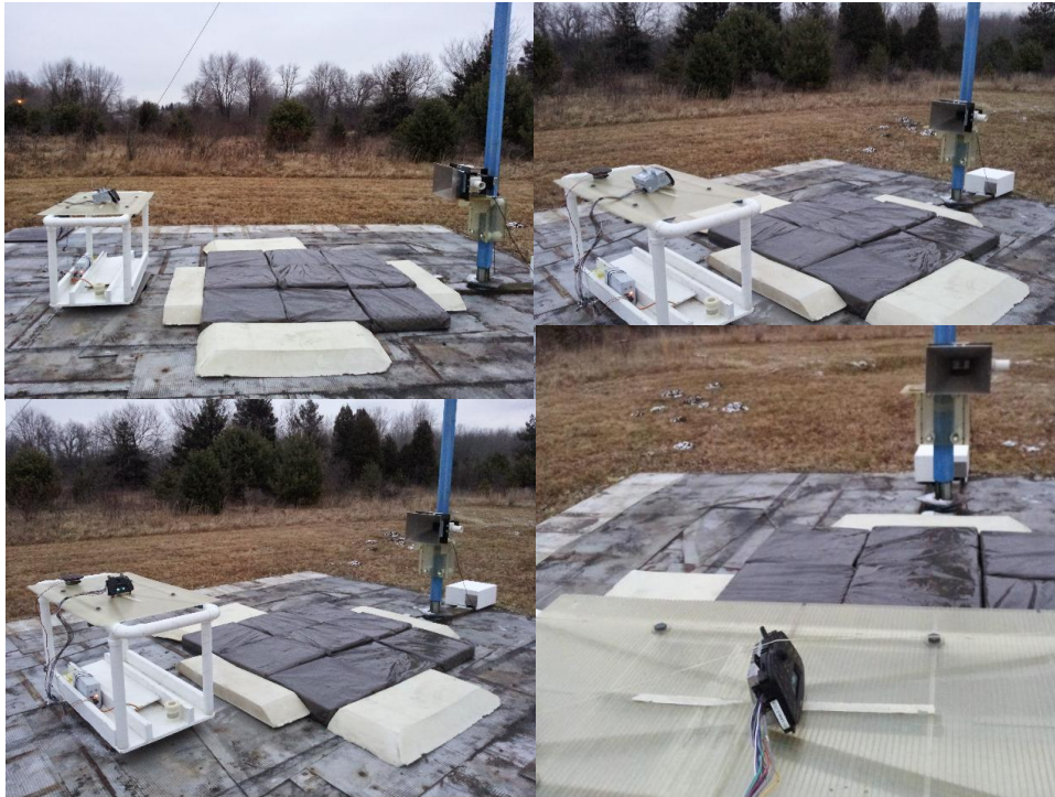
Figure 4: Radiated Emissions Test Setup Photograph(s).
