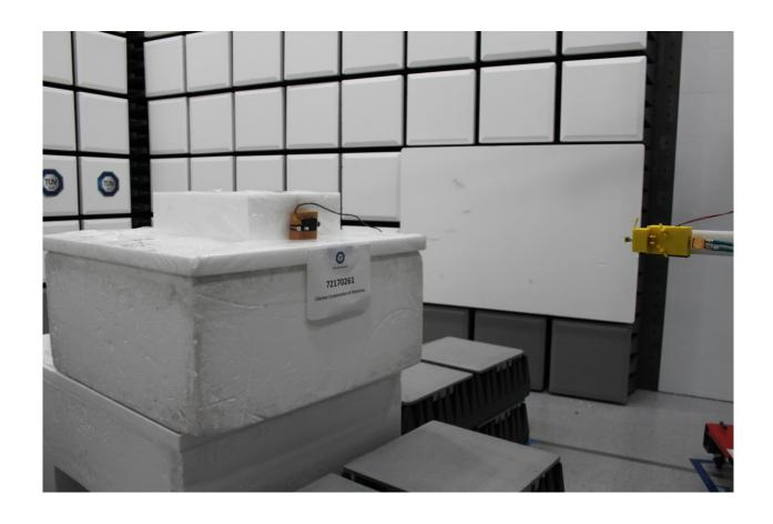
Radiated Emissions Test Setup (18GHz TO 75GHz to 140GHz)
