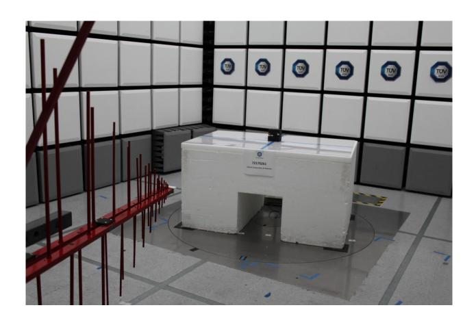
Radiated Emissions Test Setup (30MHz to 1GHz)
