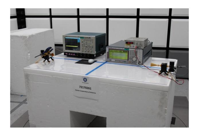
**Power Measurement/Substitution Test Setup**
