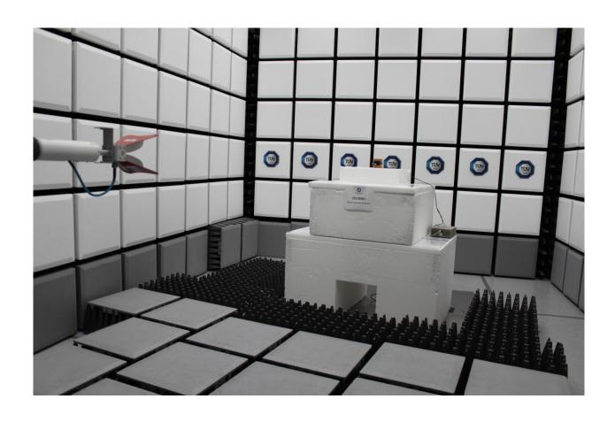
Radiated Emissions Test Setup (1GHz to 18GHz)
