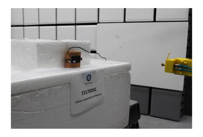
Radiated Emissions Test Setup (140GHz TO 200GHz)
