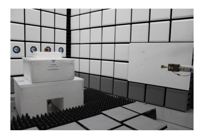
Radiated Emissions Test Setup (18GHz TO 75GHz)
