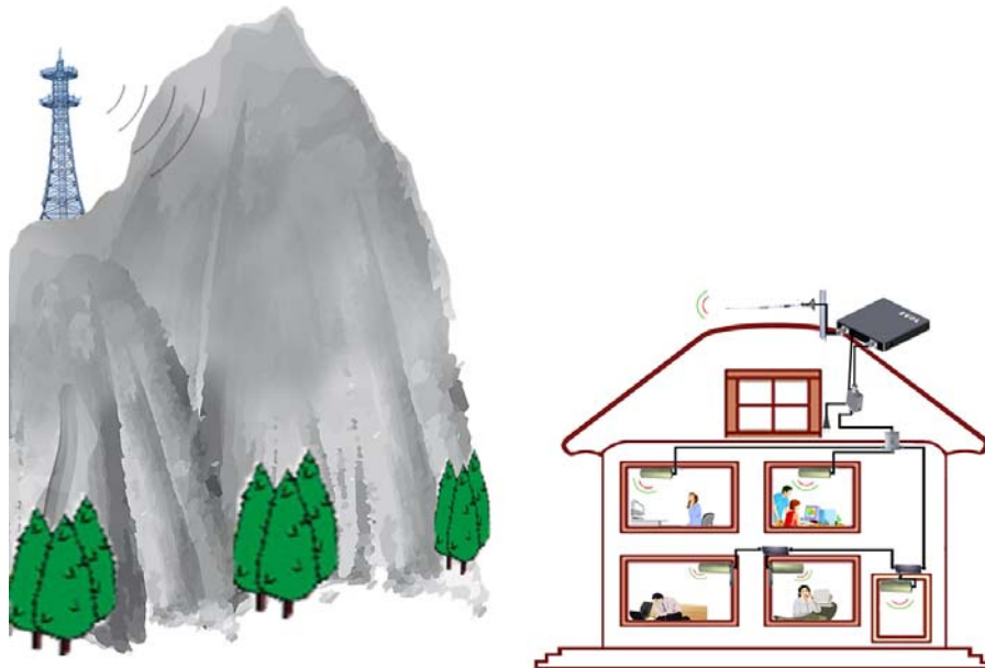
Cell phone signal amplifier communication schemes
