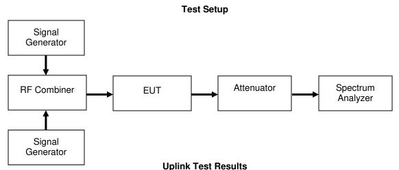
Intermod Level with Intermodulation Level **Frequency Band** Limit Result Result Input Power @ AGC (MHz) (dBm) (dBm) (Pass / Fail) + 10 dB 698 - 716 MHz -21.9-19 **Pass** -22.5 **Pass** -21 824 - 849 MHz -21.3 -19 **Pass** Pass 1850 - 1915 MHz -20.4 -19 -20.4 **Pass Pass**
