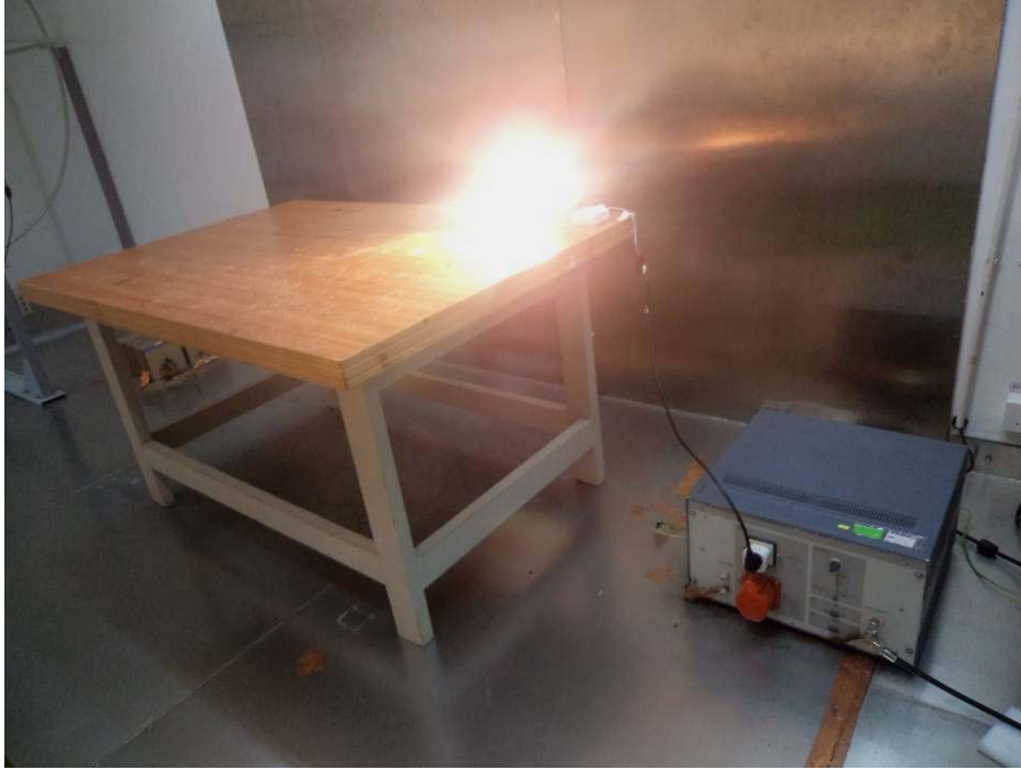
Conducted Emissions - Side View -1
