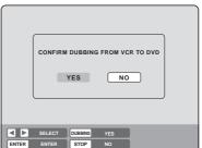
In dubbing, VCR playback, DVD recording and "dub" (dubbing) indicator appear on the display window.
