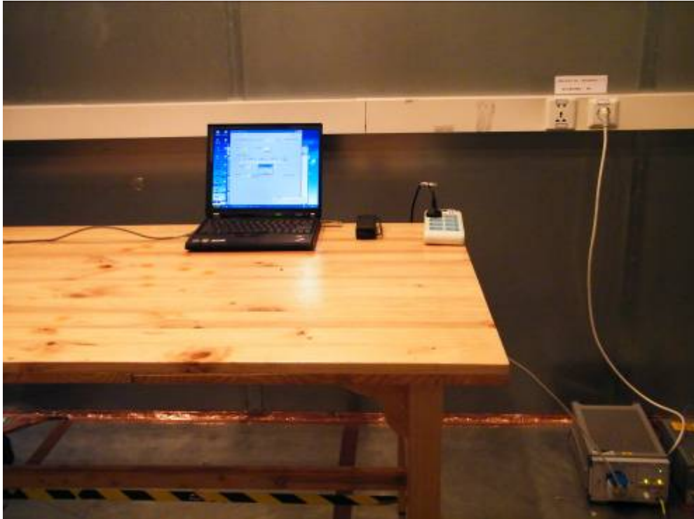
Picture 3 Conducted Emission Test Setup
