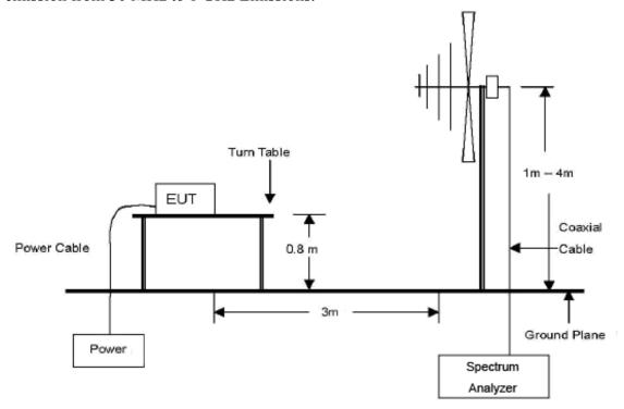
The diagram below shows the test setup that is utilized to make the measurements for emission from 1 GHz to 25 GHz Emissions.
