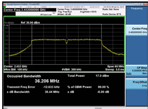
802.11n(HT40), Carrier frequency (MHz): 2452
